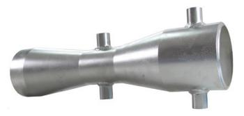
The classical venturi tube consists of a straight inlet section of the same diameter as the pipe and in which the high pressure tap is located a converging conical inlet section in which the cross section of the stream decreases and the velocity increases with a consequent increase of velocity head and decrese of pressure head.
